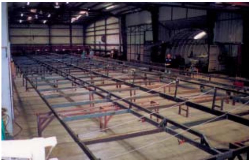
An in-depth look at a quality bi-fold door being manufactured at the Well Bilt facility in Williston, FL.
